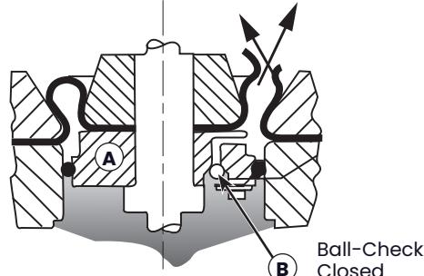
Both illustrations show the monitor in the downstream position. When installed this way, the 441-X57 is usually set for an outlet pressure 4 to 6 psi higher than the operating regulator and thus is wide open during normal operation.
